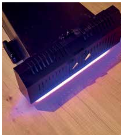
LED-CURING ON-SITE UNIT
